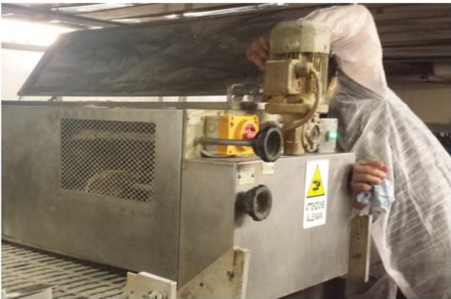
Traditional aluminum motor after 1 year working
