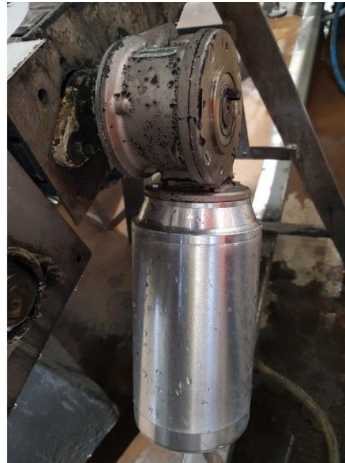
HCW motor after 2 years working in a vinegar cell and in comparison with reducer with traditional coating system
